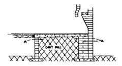
Figure 5 - Dirt Filled Step
